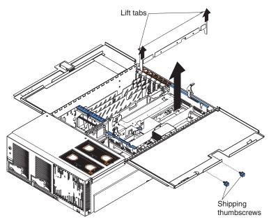
5. Remove the processor-board assembly from the server:
